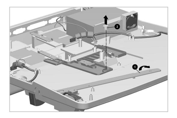
Figure 7-35. Removing the Docking Bar and Bushing
